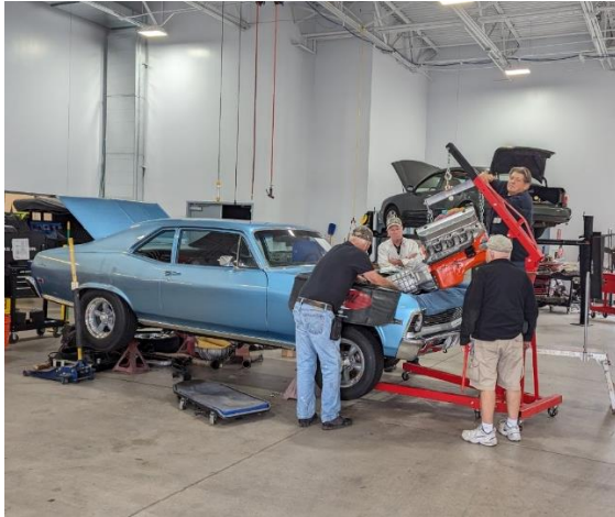
Installing Len's 454 Chev engine. Photo Courtesy of Matthew Staske.
