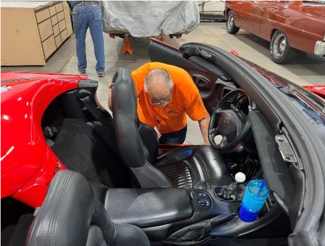
Bob Cummings putting new foam in the seats in his late model Corvette.
